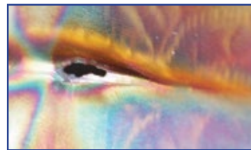
Close inspection shows a crack that separated during manufacturing.
